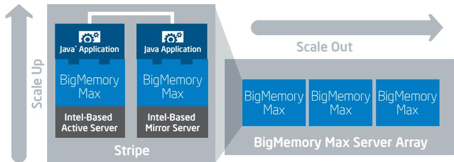
**Figure 2.** Terracotta BigMemory Max\* can pool RAM from multiple servers in an array configuration, and provides high availability and resiliency by mirroring the data across two or more servers in an array configuration
